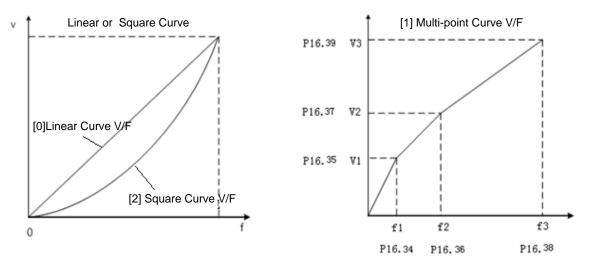
P16.34 ~ P16.45 twelve parameters define multi-point V/F curve. V/F curve is usually set based on the load characteristics of the motors. Note: V1 <V2 <V3, F1 <F2 <F3. If the set value of low-frequency voltage is too high, it may cause the motor overheat and even burn down, and the inverter stalling or overcurrent protection.
