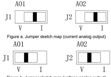
Figure b. Jumper sketch map (voltage analog output)
