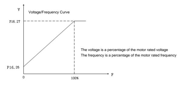
When P16.14= [2] square curve, V/F start compensating voltage setting value is p16.30. P16.30 and P16.27 can be set with reference to the following figure:
