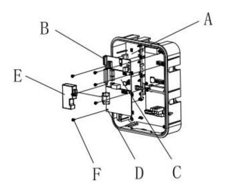
A- ground trestle B- PG card C- IO card D- DP card E- DP card adapter connector F- screw
