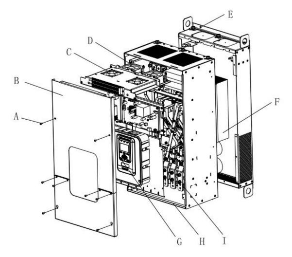
A- Cover plate bolt B- Cover plate C- Cooling fan1 D- Cooling fan2 E- Installation hole F- Radiator G- Operator H- Grille I-Main terminal
