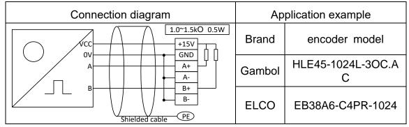
(3) Encoder output mode: voltage output
