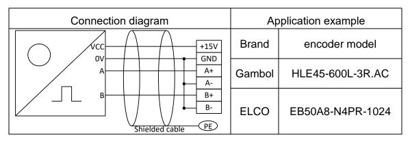
In synchronizing function application, the encoder with differential output signal wiring diagram is as follows:
