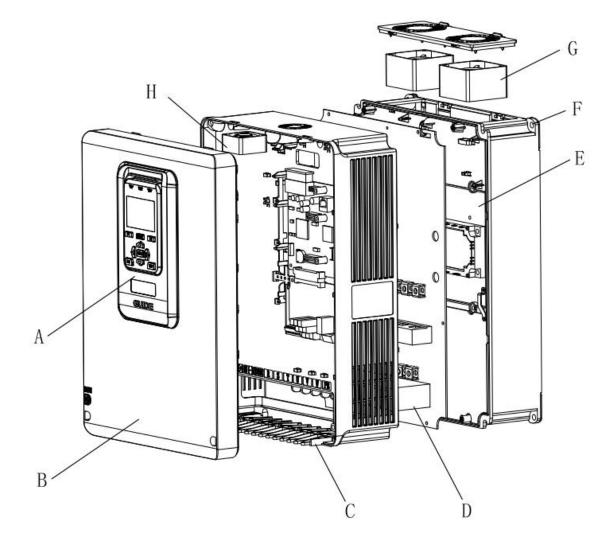
A- Operator B- Cover plate C- Grille D- Main terminal
