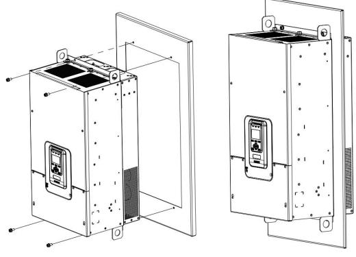
picture 3-3 inlay Installed for high-power inverter
