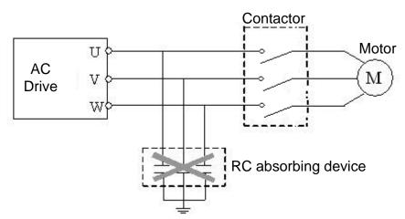
Figure 4-1 Output terminals can not be added with RC absorbing device
