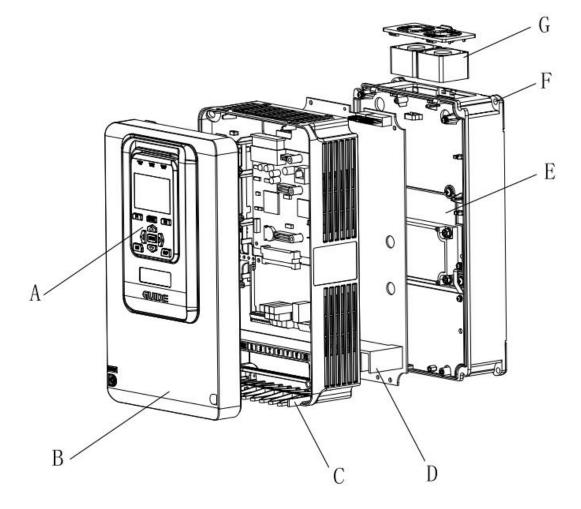
A- Operator B- Cover plate C- Grille D- Main terminal
