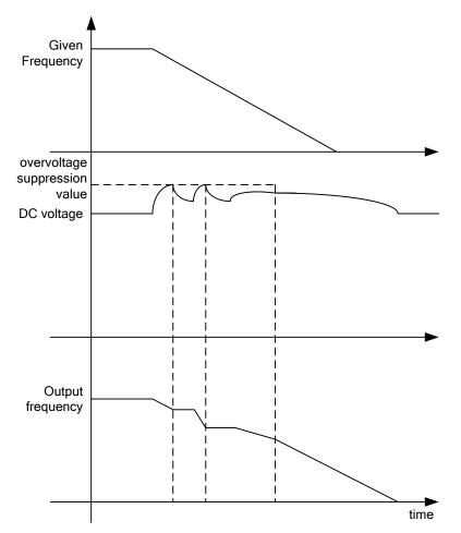
when the P7.71 is "Enable", the software will changing the motor deceleration time and increasing motor field to realize overvoltage suppression function; when the P7.71 is "Disable" the software will only changing the motor deceleration time to realize overvoltage suppression function.
