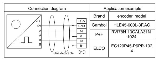
(2) Encoder output mode: open-collector output
