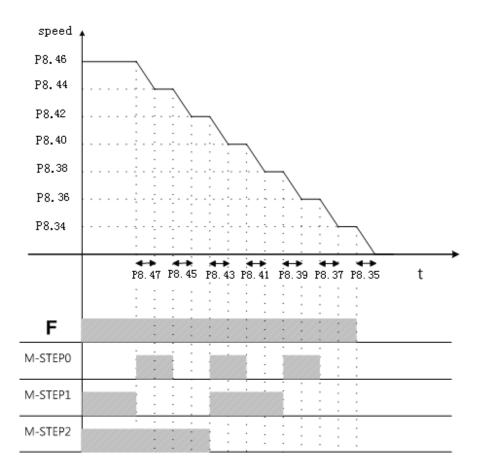
When setting the value of the deceleration region, requirement as the parameter value P8.34<P8.36<P8.38<P8.40<P8.42<P8.44<P8.46 must be obeyed, otherwise it occurs to inverter as parameter setting error.
